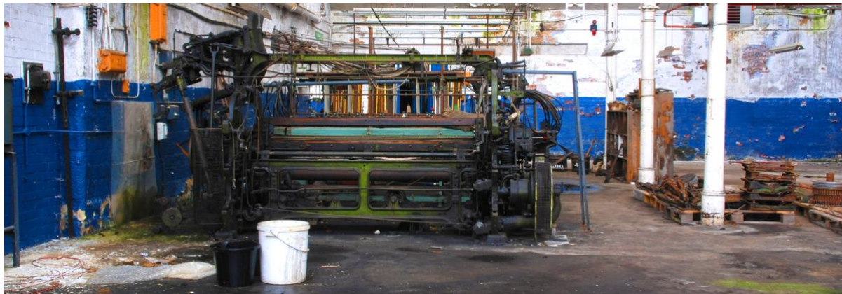
Figure 1: The Old Weaving Shed, Sunnybank Mills, with the Hattersley Loom (authors own photograph).
